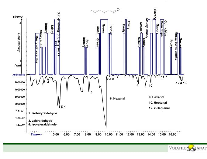
**Figure 1** An aromagram is a combination of aroma intensity vs. time (top) and a mass spectrometric total ion chromatogram (bottom). It allows for rapid screening of odorous chemicals and is useful for determining baseline volatiles and off-odors
