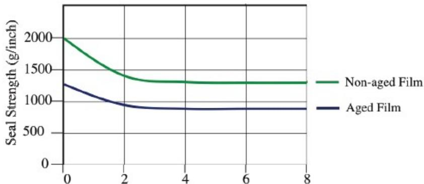
As shown in the figure above from Rollprint Packaging (Dodrill), not only is there a difference between an aged film and a non-aged film, but there is also a reduction in seal strength over time. The data illustrates that the production time line will also be a
