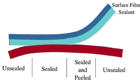
Figure 1. Adhesive Peel
