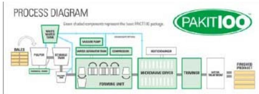
**Figure 4: PAKIT 100 Process Flow Diagram (PAKIT)**
