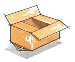
All flaps have the same length, and the two outer flaps (normally the lengthwise flaps) are one-half the container's width, so that they meet at the center of the box when folded. If the product requires a flat, even bottom surface, or the protection of two full layers, a fill-in pad can be placed between the two inner flaps.
