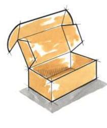
Formed from a single piece of combined board on a die cutter, the design features an unbroken bottom, several layers of corrugated in the end panels and a locking cover.
