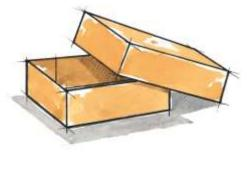
The two-piece box is made from two scored and slotted blanks (trays).
