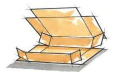
A single cut and scored piece features a fifth panel used as the closing flap, completely covering a side panel. The closed box has several layers of combined board on each end, providing stacking strength and protection for long articles of small diameter which might be damaged, or damage the box, if pushed through the ends.
