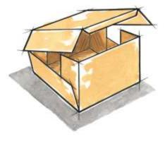
A wrap-around blank is formed into a box by folding it tightly around a rigid product. The positioning of the product, folding and sealing are performed by automatic equipment.
