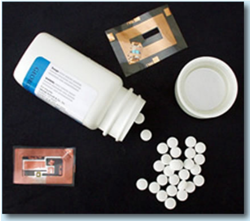
Figure 1: RFID Placed Behind Label on Pharmaceutical [5]
