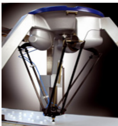
Figure 3: Delta robot, ("Robots are...," 2005)
