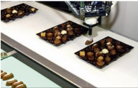
Figure 4: Pick and Place Delta robot, ("Robots are...," 2005)
